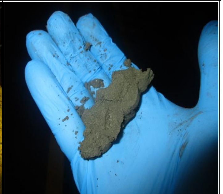
24. Grasp test indicated that no excessive moisture in cargo.
