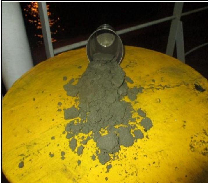
23. Can Test performed to cargo onboard observed without excessive moisture.
