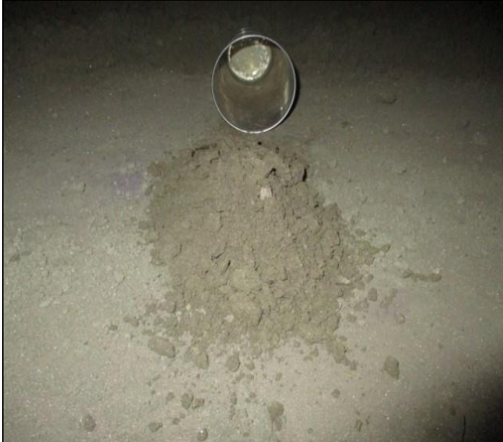
13. Can Tests performed to cargo in stockpile observed without excessive moisture.
