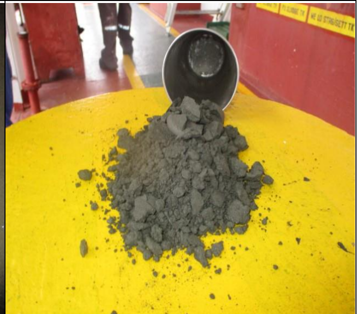
16. Can Test performed to cargo onboard observed without excessive moisture.
