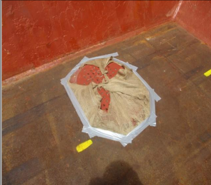
5. Hold Nr. 3, bilge well Ps, duly sealed with burlap.
