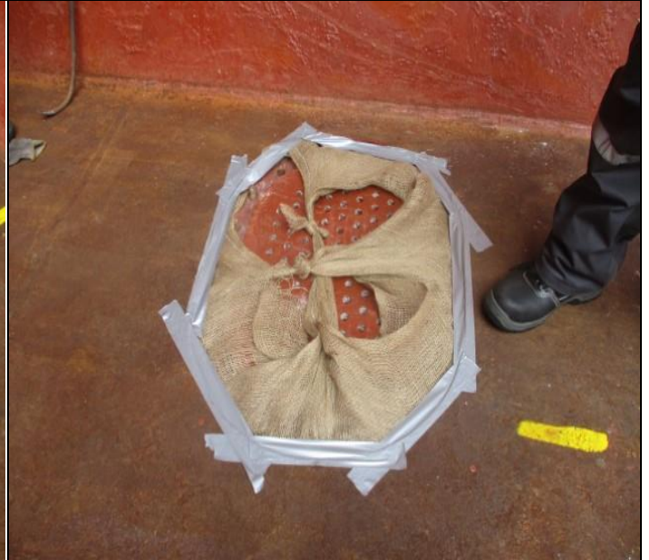
6. Hold Nr. 3, bilge well Ss, duly sealed with burlap.
