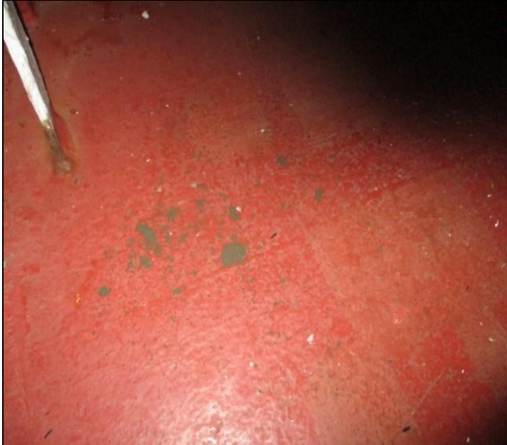
25. Drop test without signs of excessive moisture in cargo.
