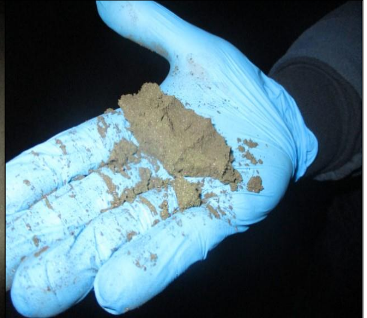
14. Grasp test carried out to cargo inside stockpile.
