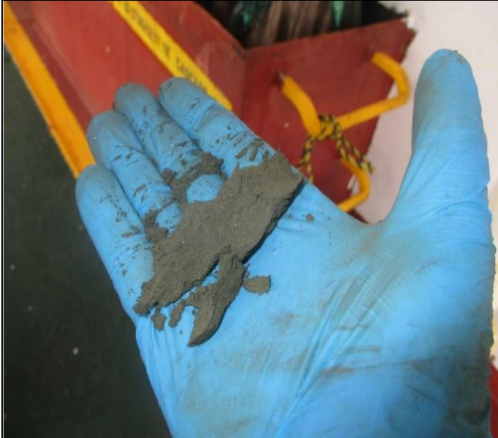
17. Grasp test indicated that no excessive moisture in cargo.
