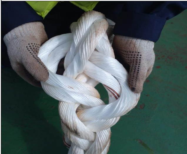
7. Internal condition of the ropes.
