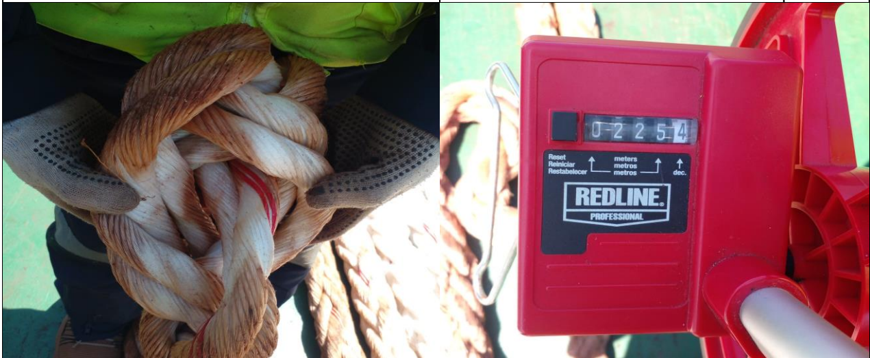
31. Internal condition of the ropes.
