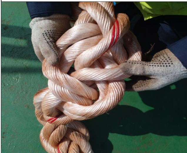
23. Internal condition of the ropes
