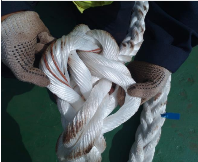
15. Internal condition of the ropes.
