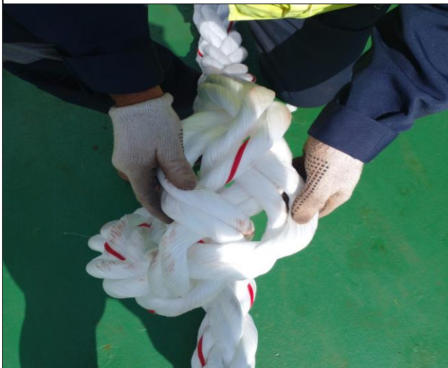
27. Internal condition of the ropes.
