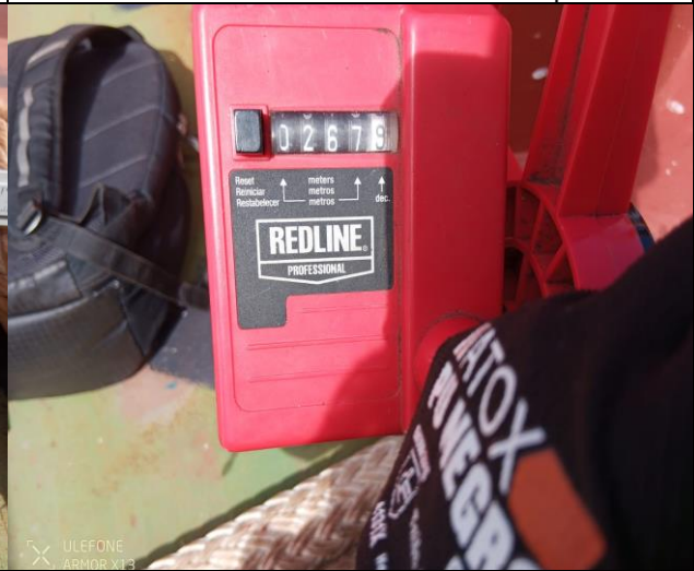
12. Length measured by surveyor.
