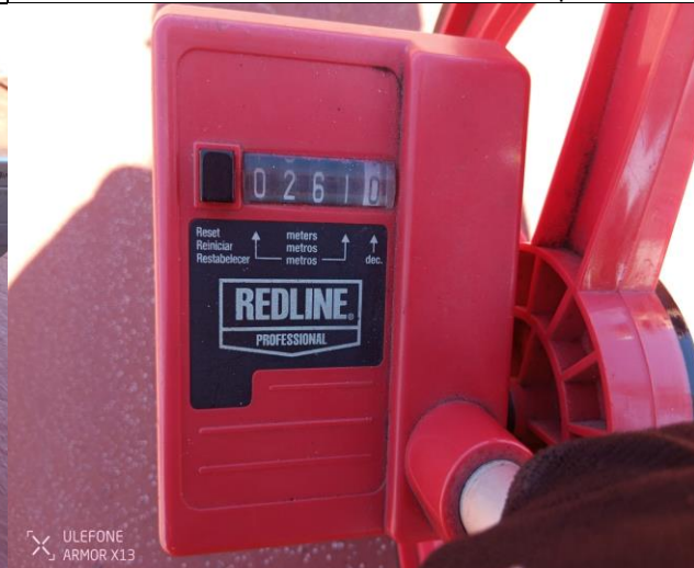
60. Length measured by surveyor.
