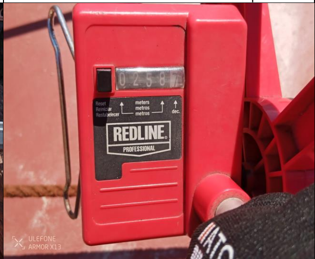
48. Length measured by surveyor.
