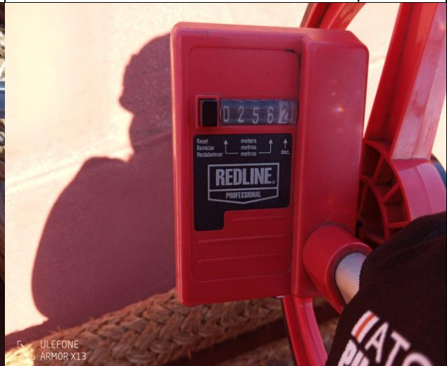
52. Length measured by surveyor.
