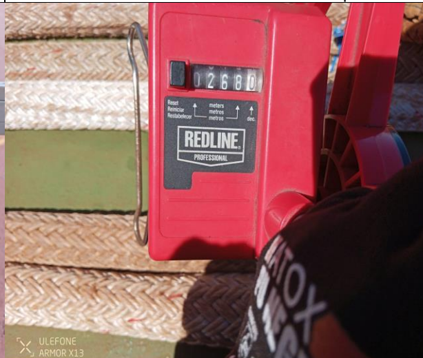
28. Length measure by surveyor.
