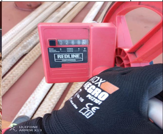
24. Length measure by surveyor.
