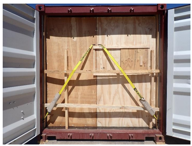
42. View of lashing of container using polypropylene sling and wooden.
