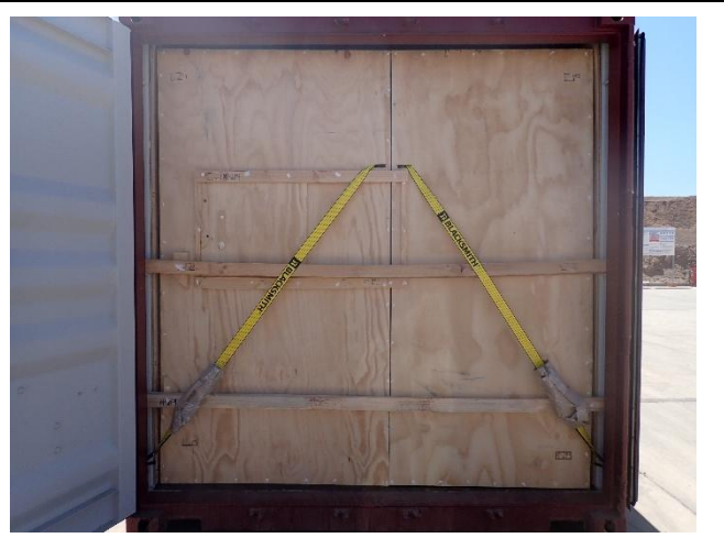
58. View of lashing of container using polypropylene sling and wooden.
