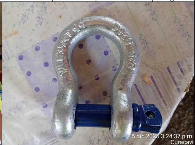
8. Shackles used to fit the sling hooks on container ringbolts.
