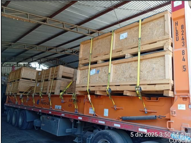
11. Final view of cargo storage and lashed over the container.
