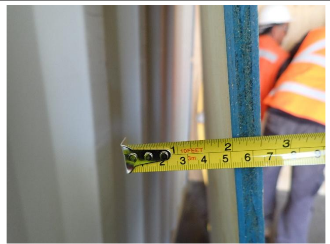
16. Measure of wood 12 mm.
