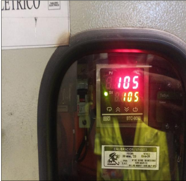
36. Oven temperature of 105.0 °C.
