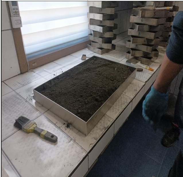
30. Sample being divided by AHK Lab personnel.
