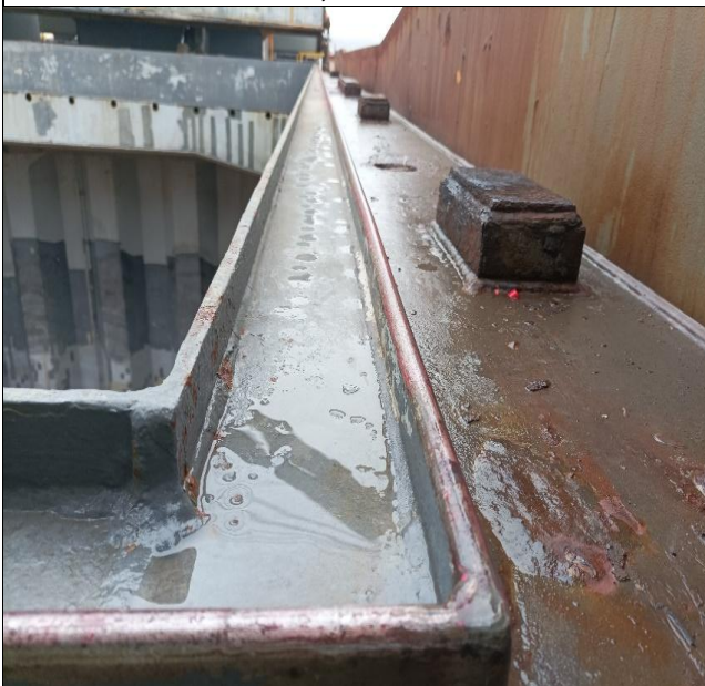
14. Hold Nr. 2, compression bar in good conditions.
