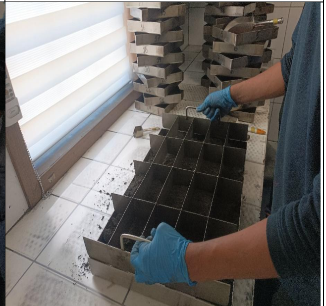
31. Sample divided in 20 square portions for filling the tray.
