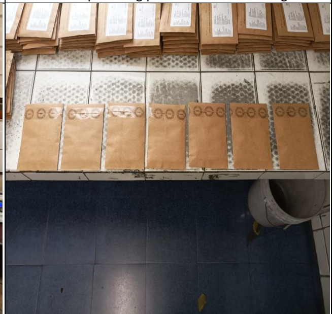
43. Samples into kraft bags sealed with AHK tape by laboratory personnel.
