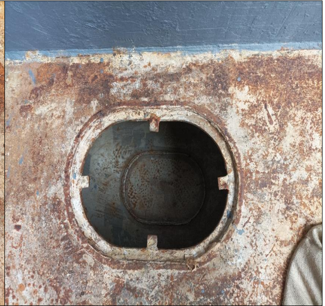
9. Hold Nr. 2, bilge/Ss clean and dry.
