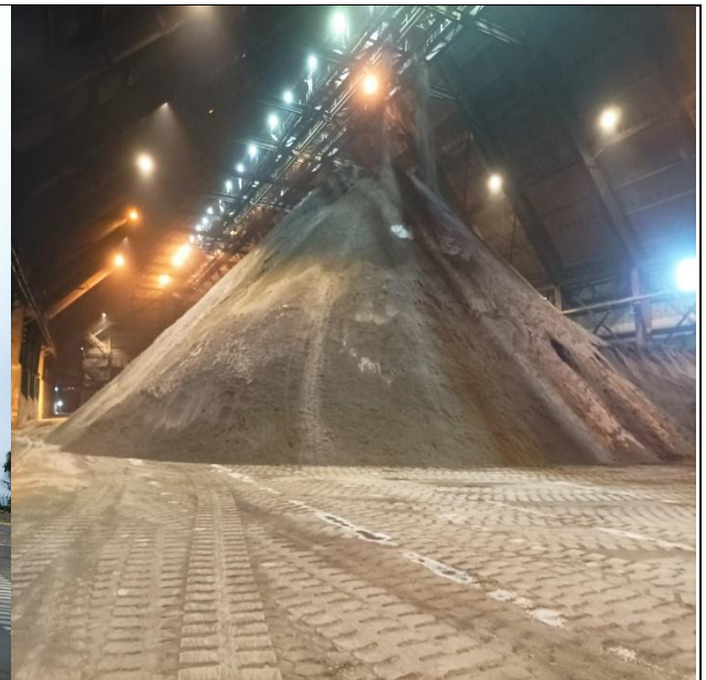
19. Copper concentrate inside stockpile prior commencement of loading operation.
