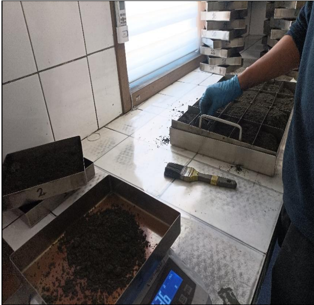
32. Sample being put into tray.
