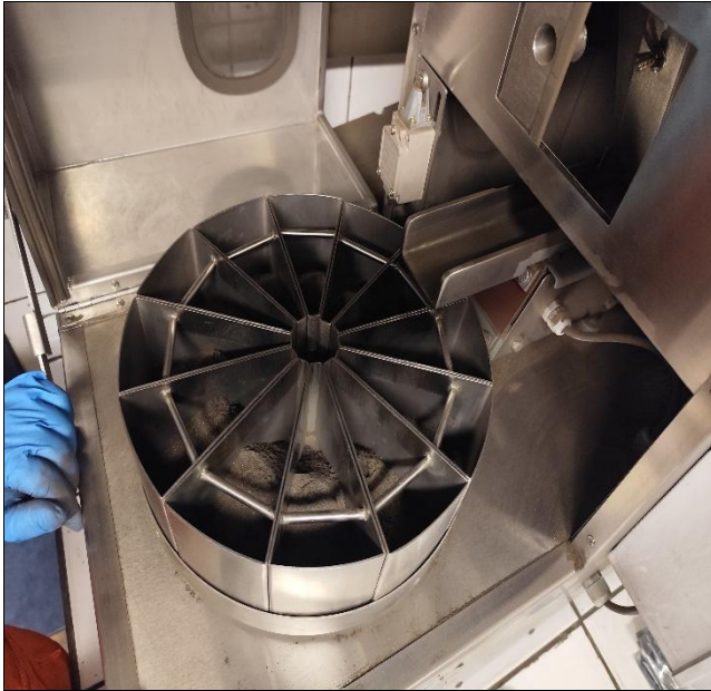
40. Dried sample into automatic divider.
