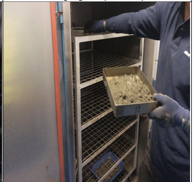
35. Trays with samples into the oven.
