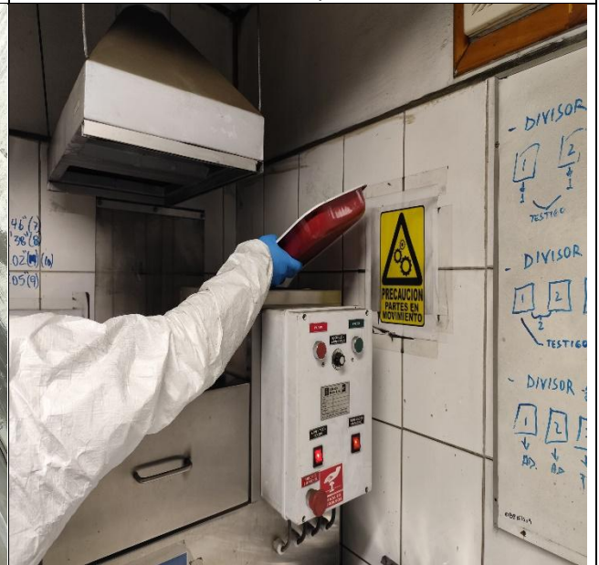
39. Dried sample being put into automatic divider.
