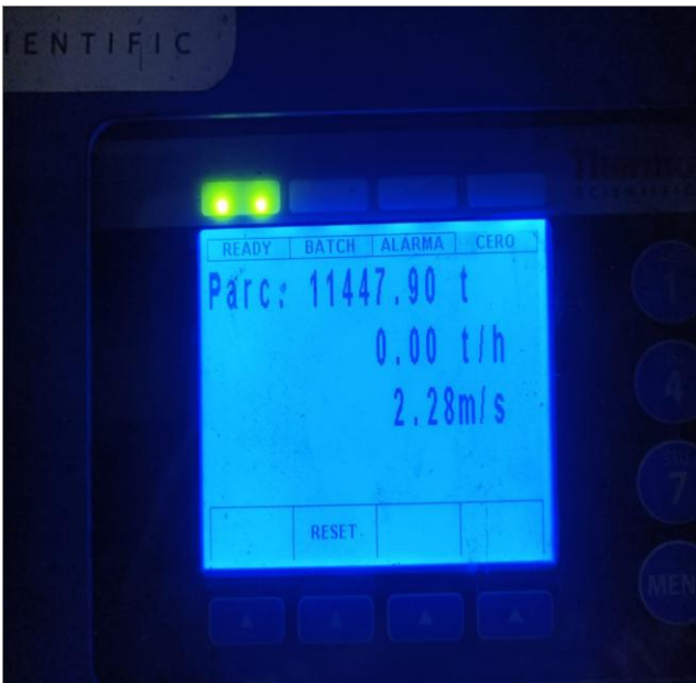
26. Weighing scale before commencing loading operation in hold Nr. 2.
