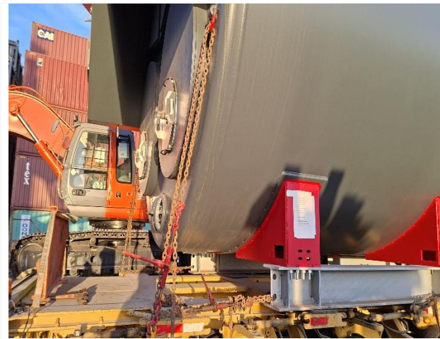
17. Cargo loaded onto the truck and lashed with chains
