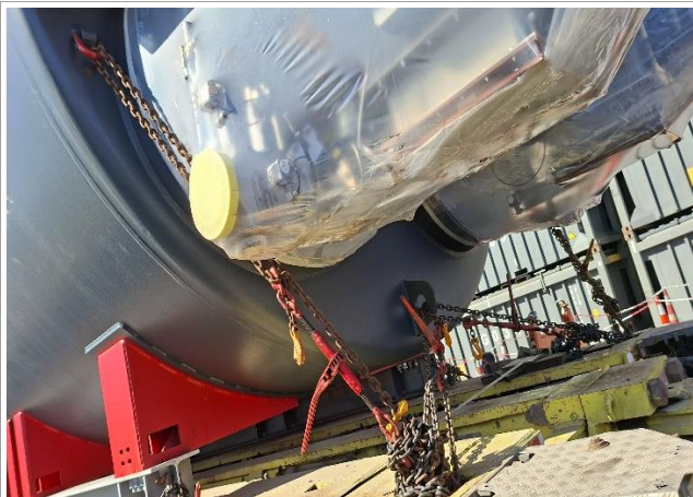
11. Cargo lashed made fast to truck ringbolt
