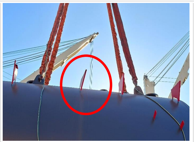
6. Frame reinforcement bent
