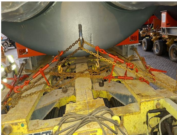
23. Bolier lashed with chains made fast to truck rignbolt
