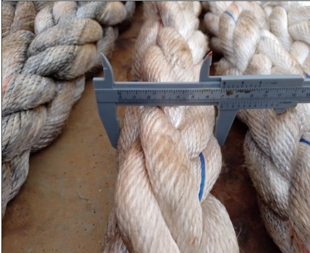
26. Diameter of the mooring line.
