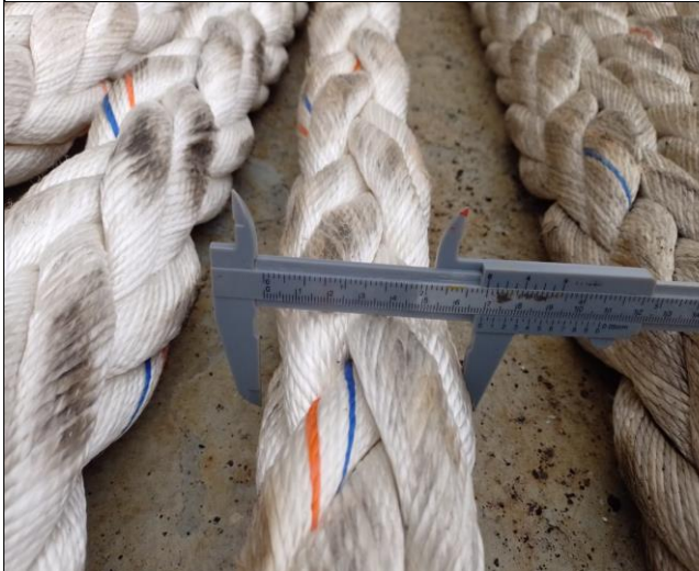
3. Diameter of the mooring rope.
