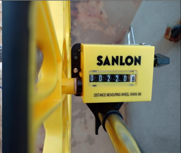
27. Length measure by surveyor.
