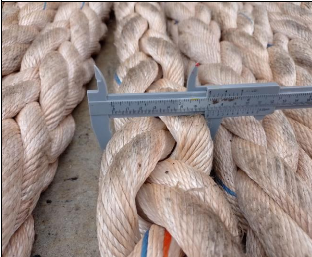
22. Diameter of the mooring rope.
