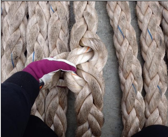
10. Internal view of ropes.
