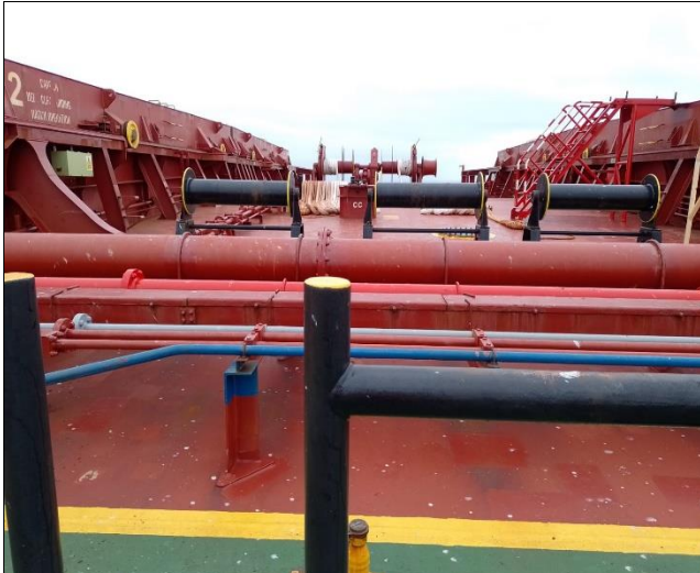
45. View of spring Btw 3-2 Pedestal Roller Guide.
