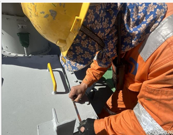
7. Painting ruler before sounding ballast.
