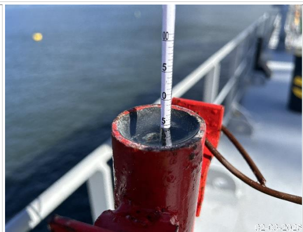
8. Checking density of the sea water.
