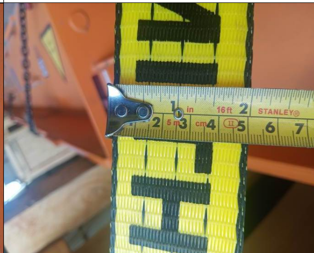
4. Slings thickness of 50mm.
