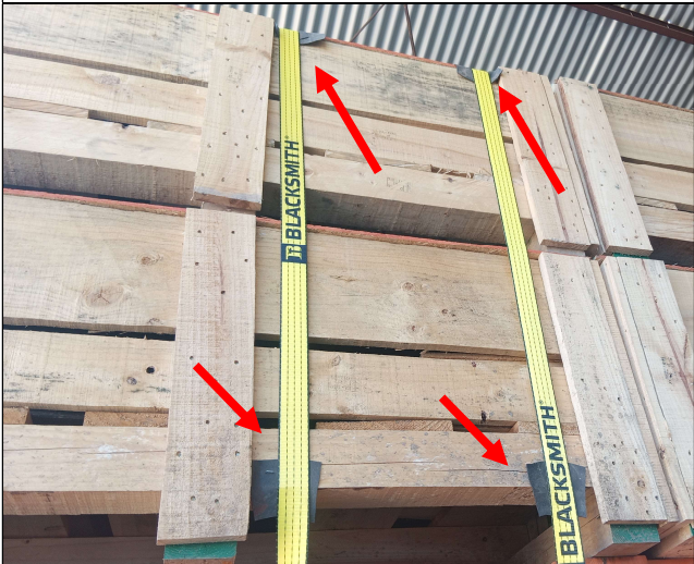
7. Rubber protection places on sharp edges.
