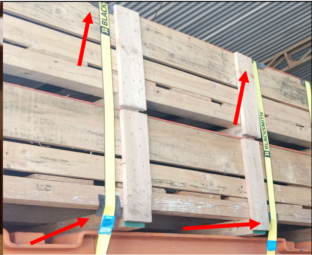
6. Rubber protection places on sharp edges.
