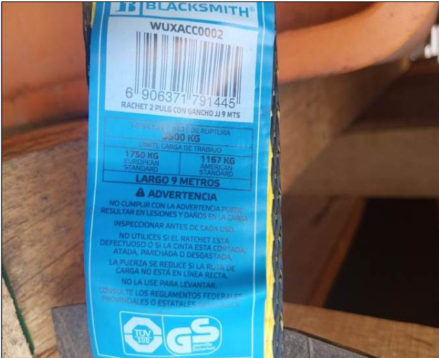
5. Sling capacity, 1750 kg WLL.
