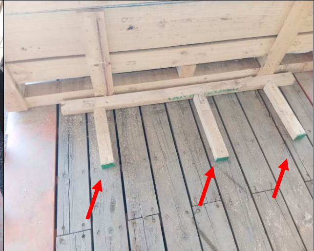
10. Crates were checked by means square lumbers.
