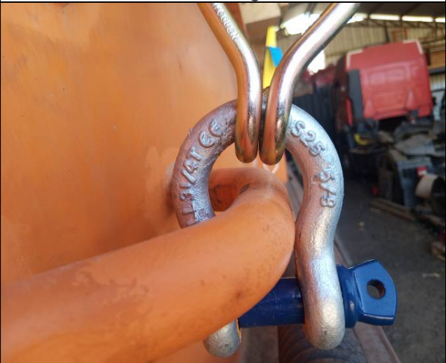
8. Shackles of 5/8 used to fit the sling hooks on container ringbolts. WLL 3 ¼ ton.
