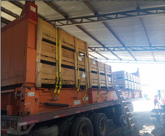
13. Final view of cargo stowage and lashed over the container.
