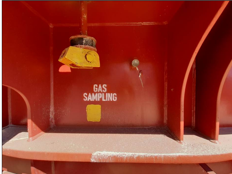
41. Hatchcover No. 2, active cleat in good conditions.
