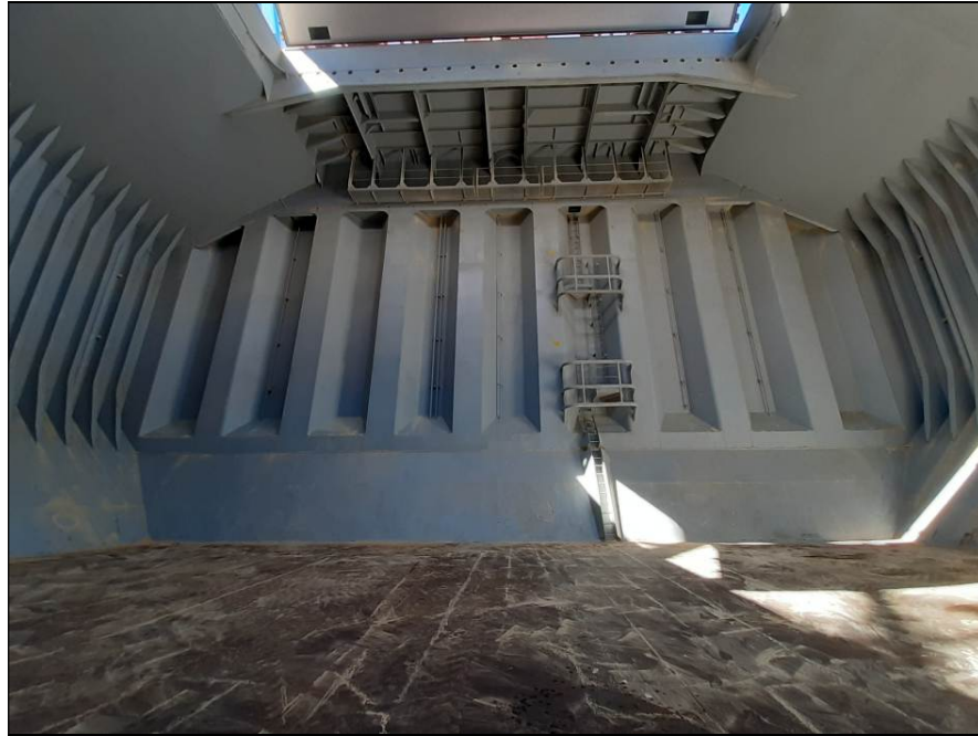
47. Aft bulkhead, with paint scratched and dust.
