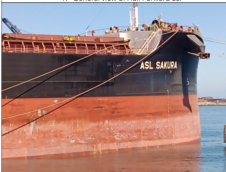
2. Paint scratched and stained were observed at fwd.
