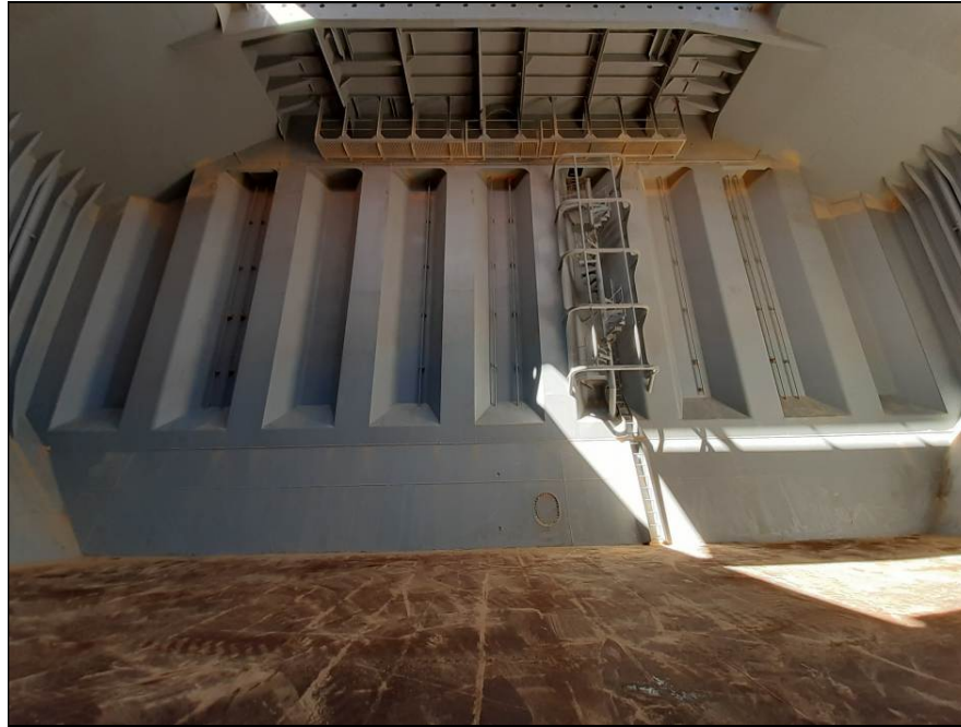
29. Aft bulkhead with paint scratched and dust.
