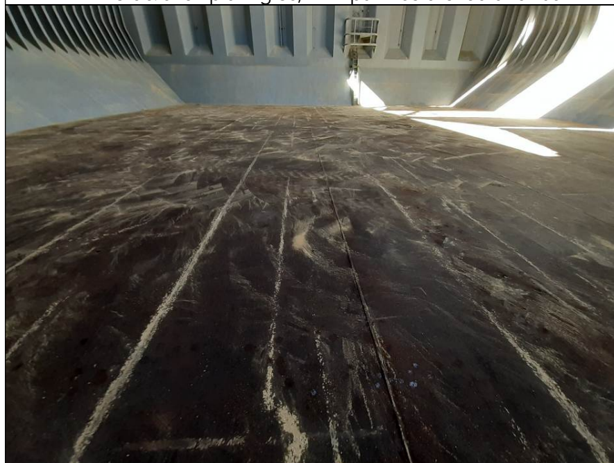
50. Tank top plating with dust of cargo discharged.
