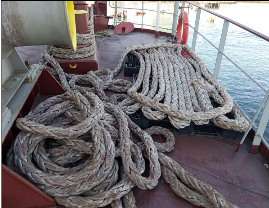
25. Aft mooring lines stained and worn out.
