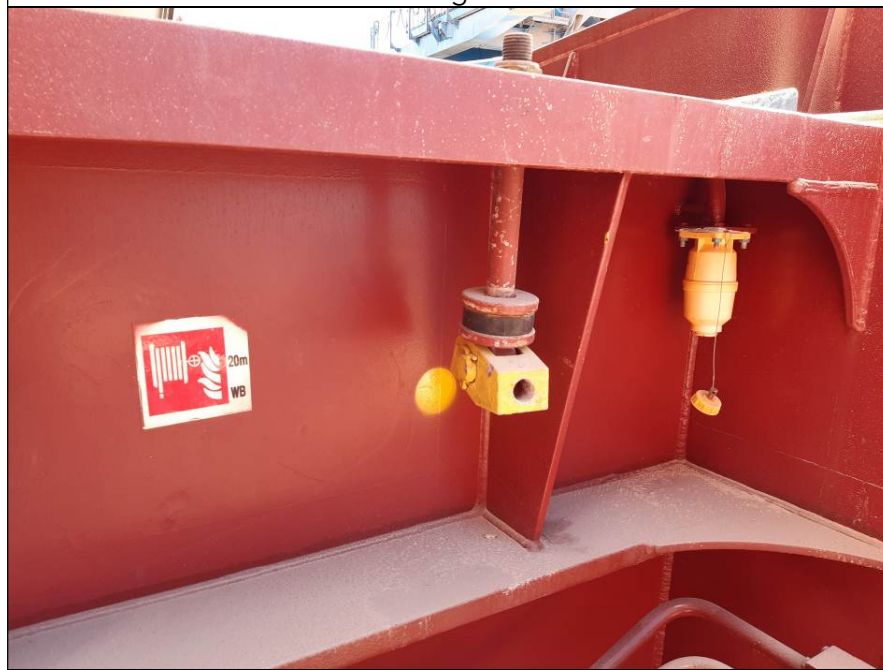
52. Hatchcover No. 3, non-return valves & acting cleats in good conditions.
