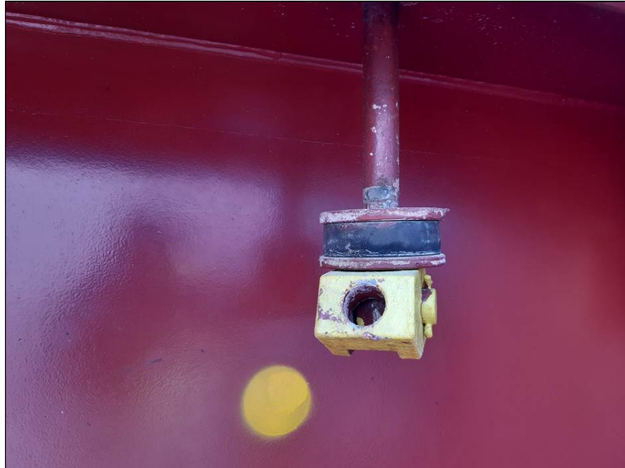
71. Hatchcover No. 5, active cleats valves in good conditions.
