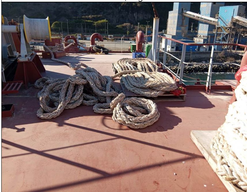
20. Forward mooring lines stained and worn out.
