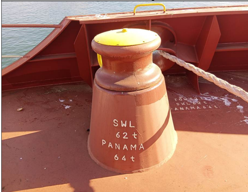
16. Roller guides in good conditions.
