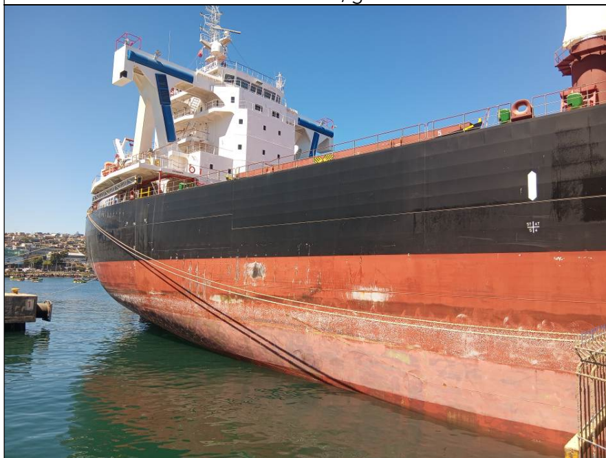
10. Hull with paint scratched & stained.
