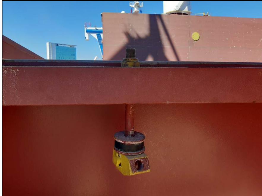
61. Hatchcover No. 4, active cleats valves in good conditions.
