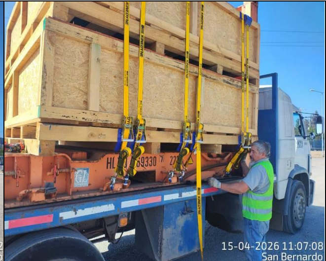
6. Lashing operations with slings.
