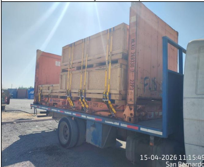
15. Final view of cargo lashed over the container.
