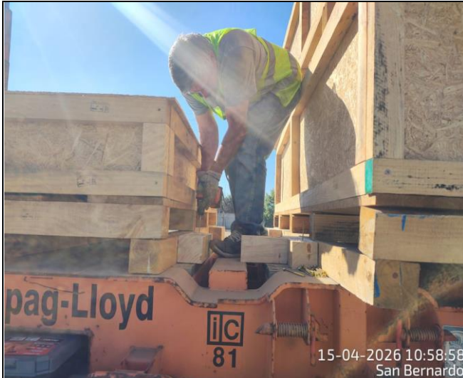
13. Crate chocked by means square lumbers.
