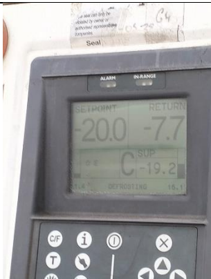
Frozen Unit : Set point - 20.0 °C, Supply Tempertature -19.2°C, Return Temperature -7.7 °C
