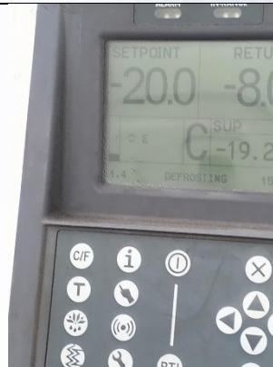
Frozen Unit : Set point - 20.0 °C, Supply Tempertature -19.2°C, Return Temperature -7.7 °C
