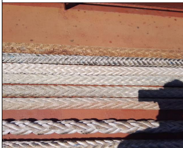
3. Another view of mooring lines arranged for its inspection.
