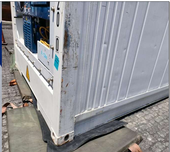
12. 1x40' RF HC HLBU 617420-0, left panel, with scratches on paint coating.
