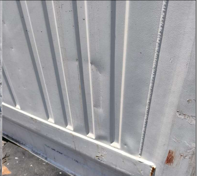
10. 1x40' RF HC HLBU 617420-0, left panel with scratches and dented. Section 1 lower part
