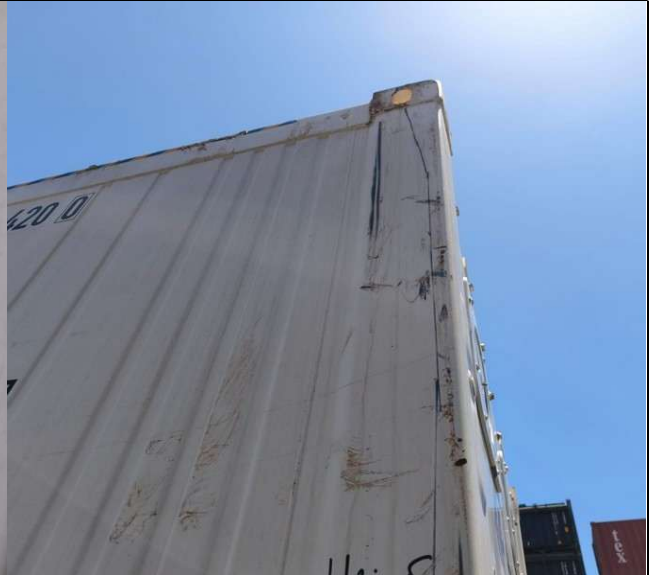
14. 1x40' RF HC HLBU 617420-0, right panel, with scratches on paint coating.
