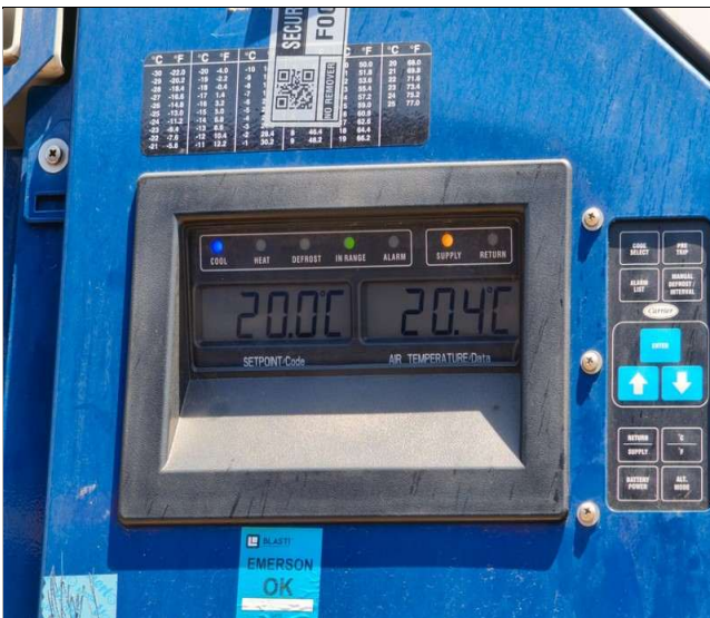
23. 1x40' RF HC HLBU 617420-0 setting temperature to 20°.
