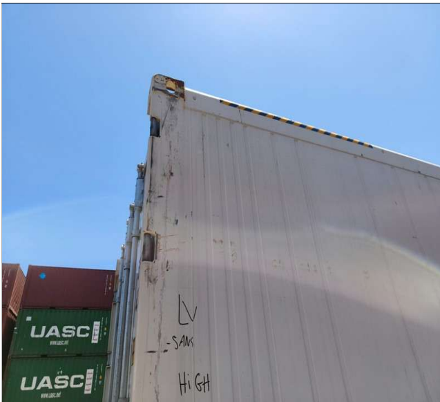
15. 1x40' RF HC HLBU 617420-0, right panel, with scratches on paint coating.
