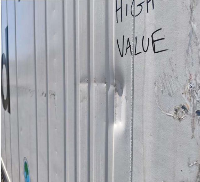
9. 1x40' RF HC HLBU 617420-0, left panel with scratches and dented. Section 1 middle part.
