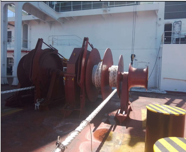
3. General view of rope located onto drum
