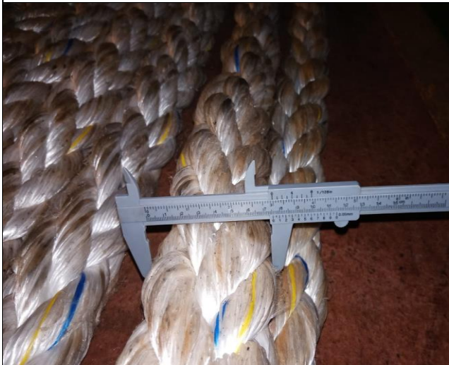
27. View of diameter measurement of the mooring lines.
