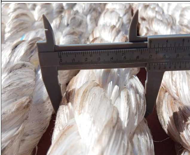
7. View of diameter measurement of the mooring lines.
