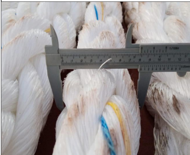
31. View of diameter measurement of the mooring lines.
