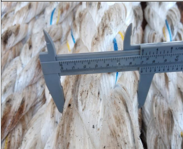
19. View of diameter measurement of the mooring lines.
