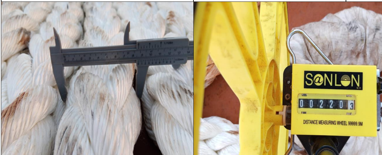
39. View of diameter measurement of the mooring lines.
