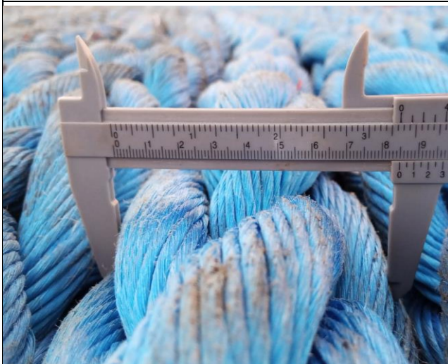
15. View of diameter measurement of the mooring lines.
