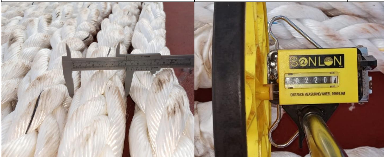
35. View of diameter measurement of the mooring lines.
