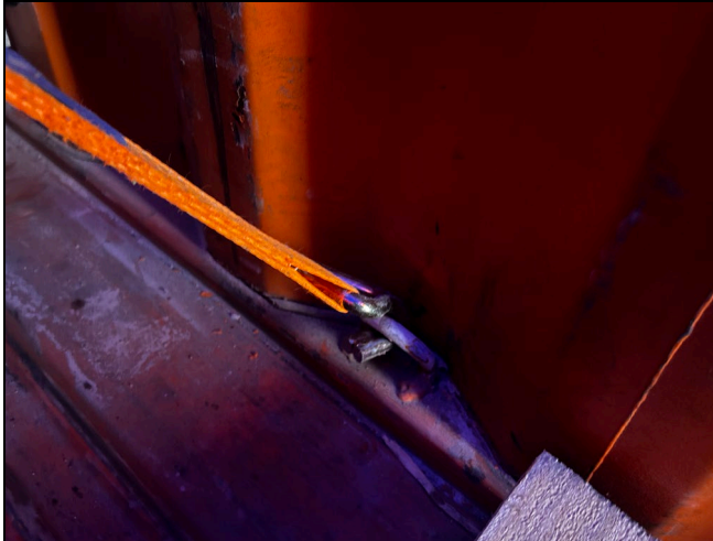
9. View of lashing conditions, hook located in container d-ring
