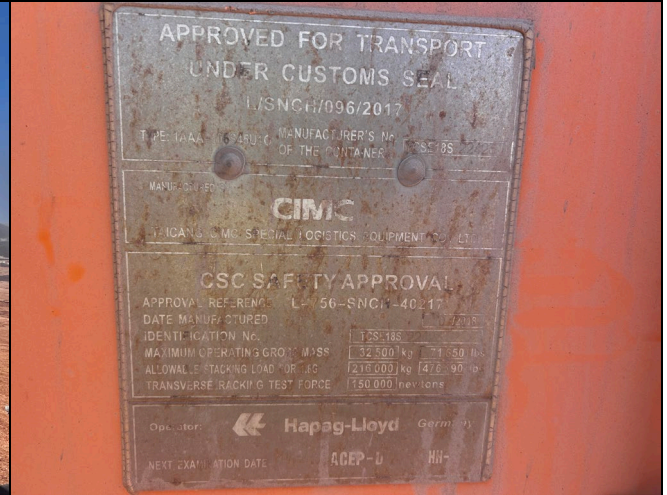
2. CSC Plate in good conditions
