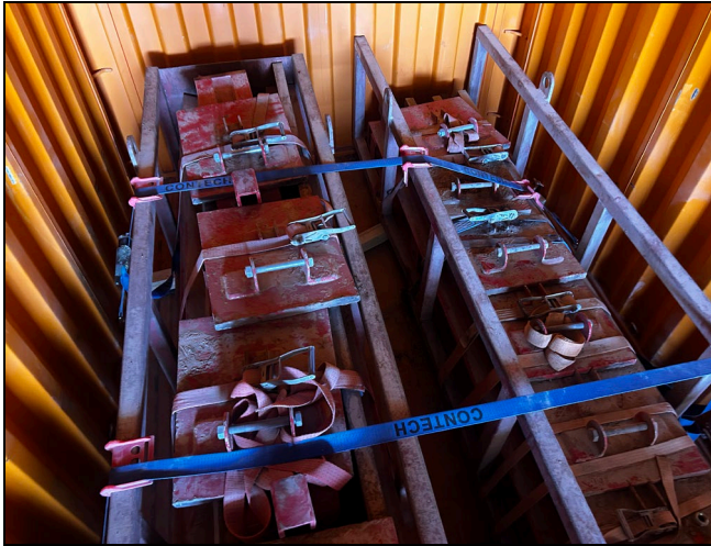
5. View of lashing bands and rubber protection
