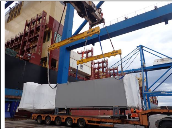
First lifting in which was observed that the lifting will be not horizontally
