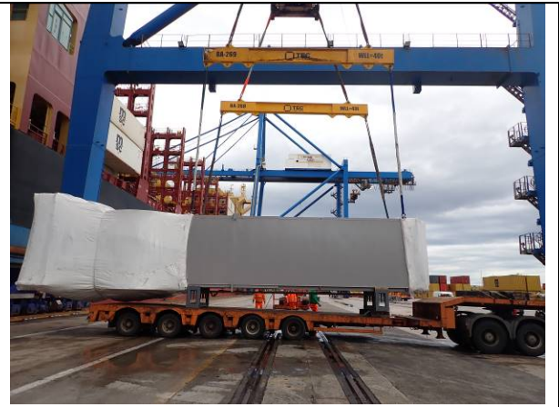
First lifting in which was observed that the lifting will be not horizontally
