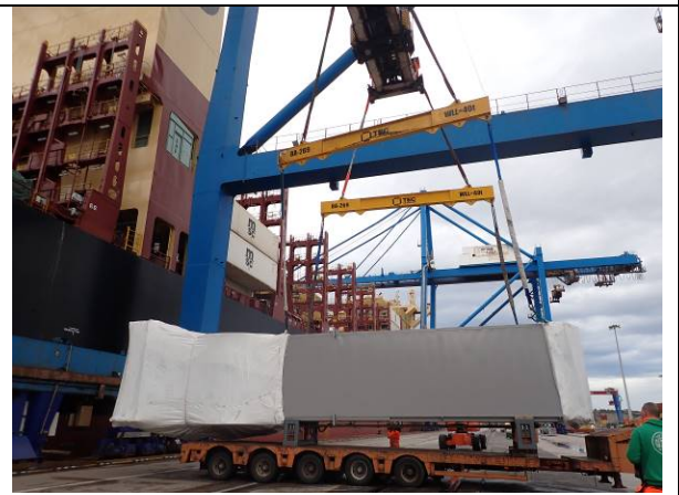
Lifting with rigging modified and correct
