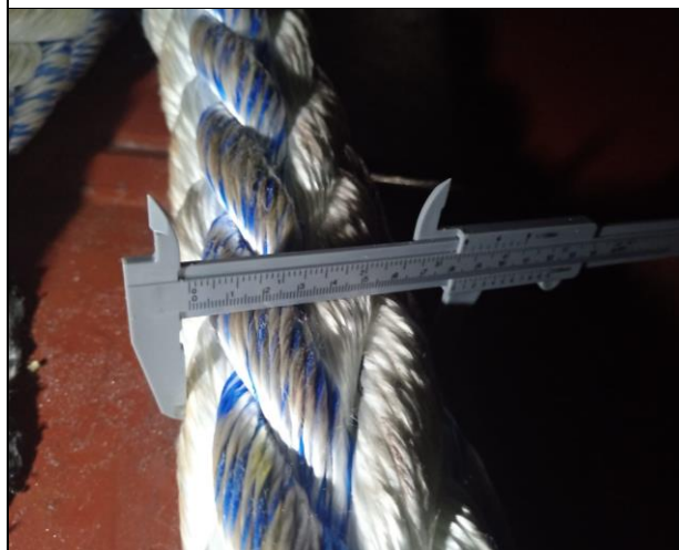
3. View of diameter measurement of the mooring lines.
