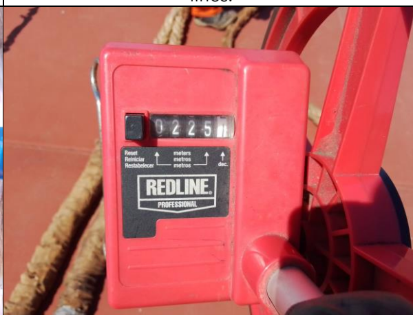
7. View of length measurement of mooring lines.
