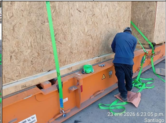
8. Cargo being chocked with square lumbers.
