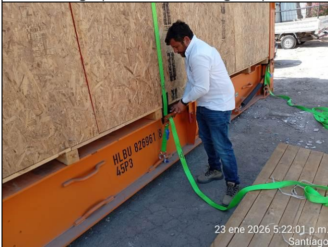
7. Lashing operation with slings in process.
