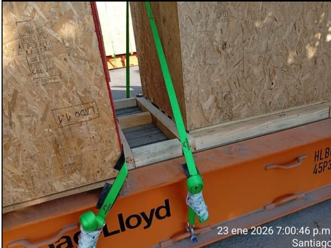
9. Wooden crates chocked with square lumbers and with rubber pieces at the edges.
