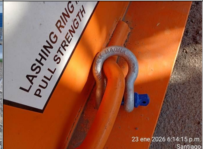
12. Shackle with a capacity WLL of 4.75 Tons.
