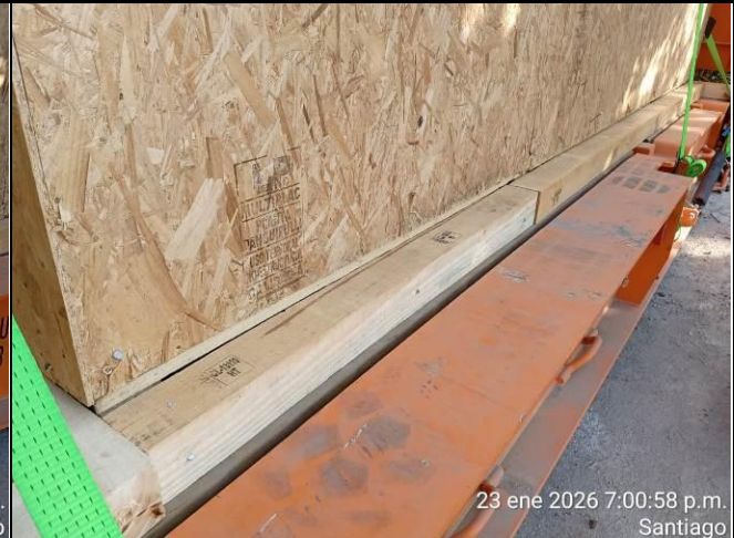
10. Square lumbers used for to avoid shifting wooden crates with ISPM -15 stamp.
