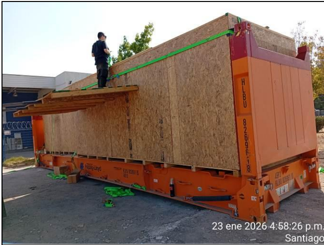
5. Lashing operation with slings in process.
