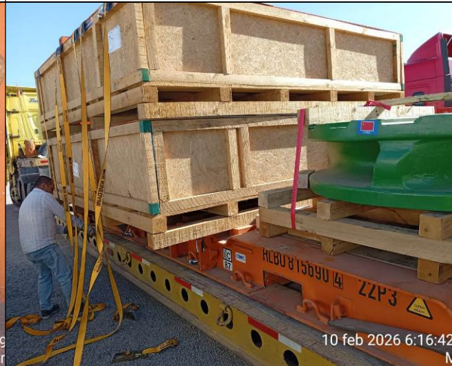
4. Lashing operations with slings.
