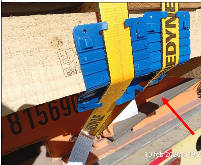
7. Plastics protections placed between slings and sharp edges.
