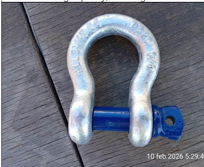
11. Shackles used to fit the sling hooks on container ringbolts.
