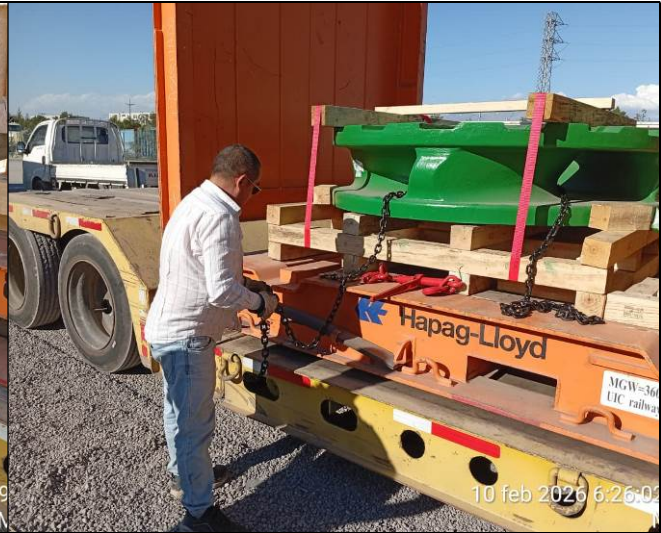
6. Lashing operations with steel chains.
