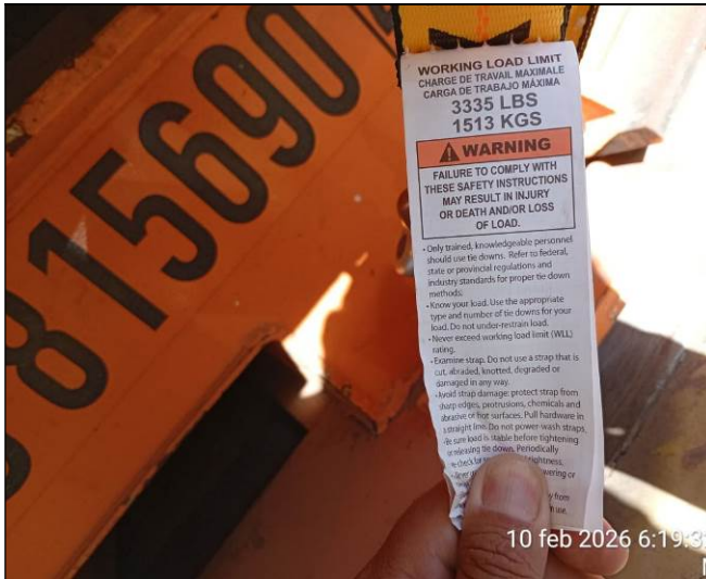
9. Sling capacity, 1513 Kg SWL.
