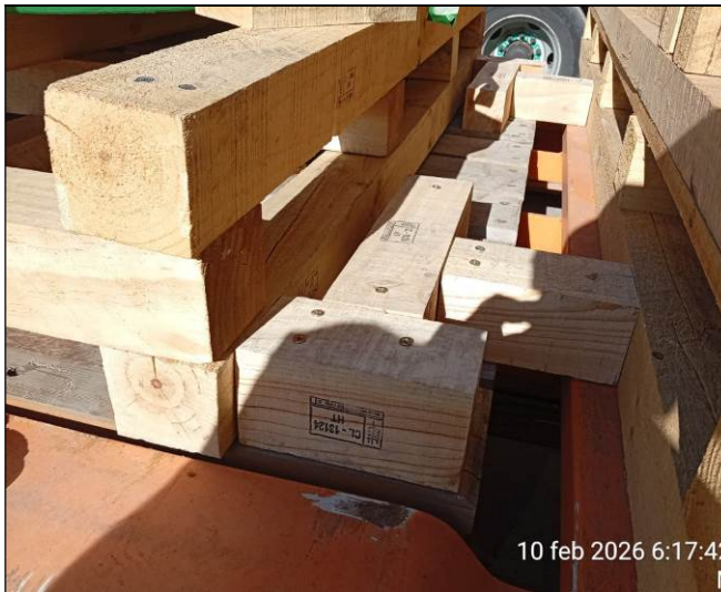
13. Crate chocked by means square ladders.
