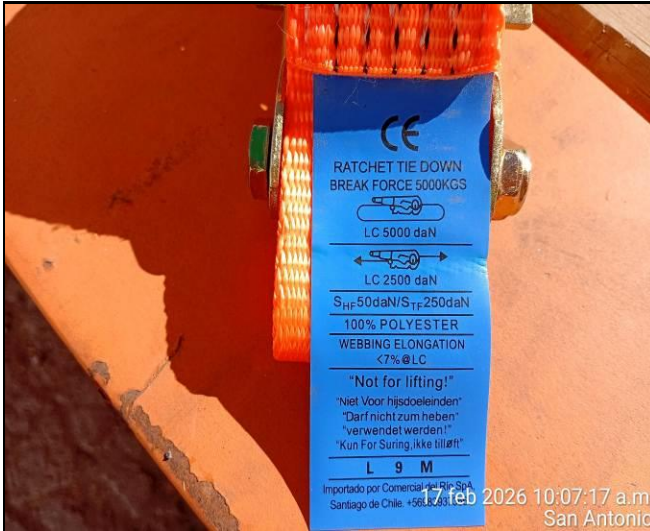
9. Sling capacity, LC 2500 Kg.
