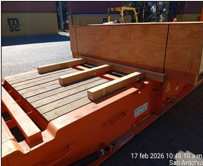
13. Crate chocked by means square ladders.
