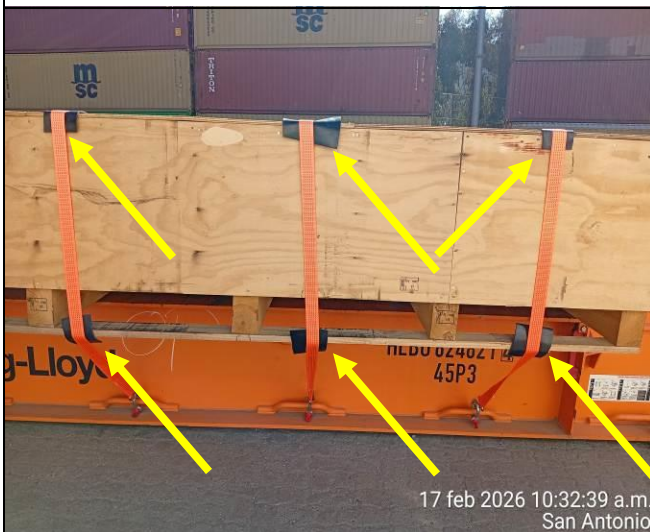
7. Rubber protections placed between slings and sharp edges.
