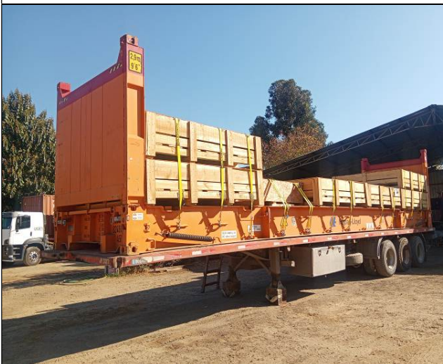
15. Final view of cargo stowage and lashed over the container.
