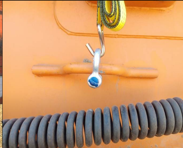
10. Shackles used to fit the sling hooks on container ringbolts.
