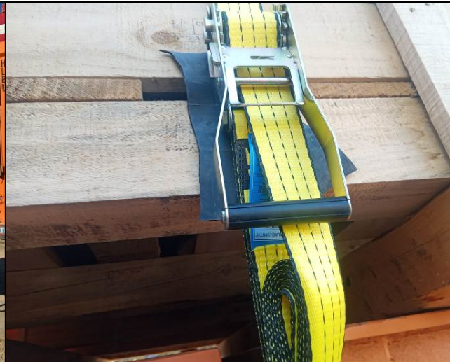
6. Rubber protections placed on sharp edges.
