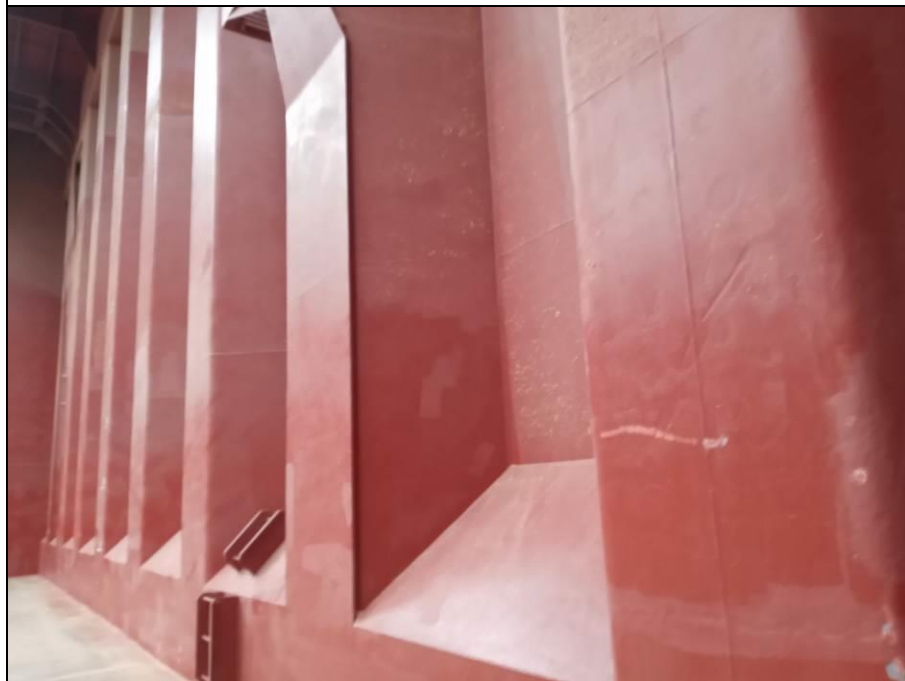
68. Fwd bulkhead with paint scratched.
