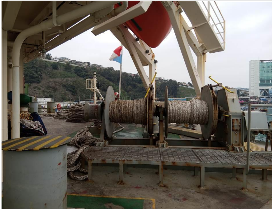
23. Winch Ps poop deck, in good conditions.
