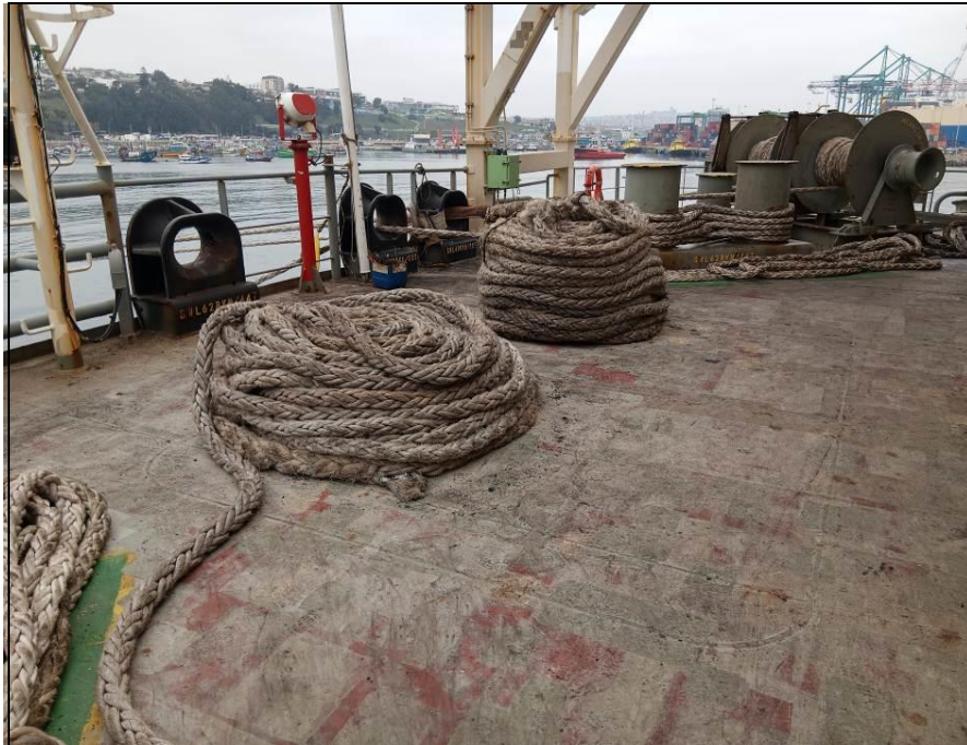
25. Aft mooring lines stained and worn out.
