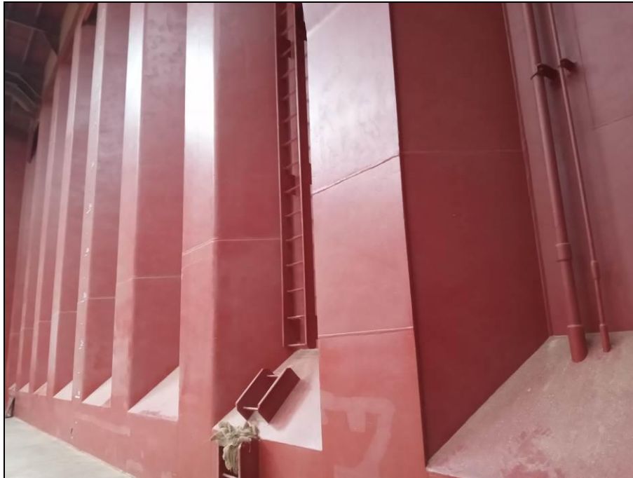
39. Aft bulkhead, with paint scratched and dust.
