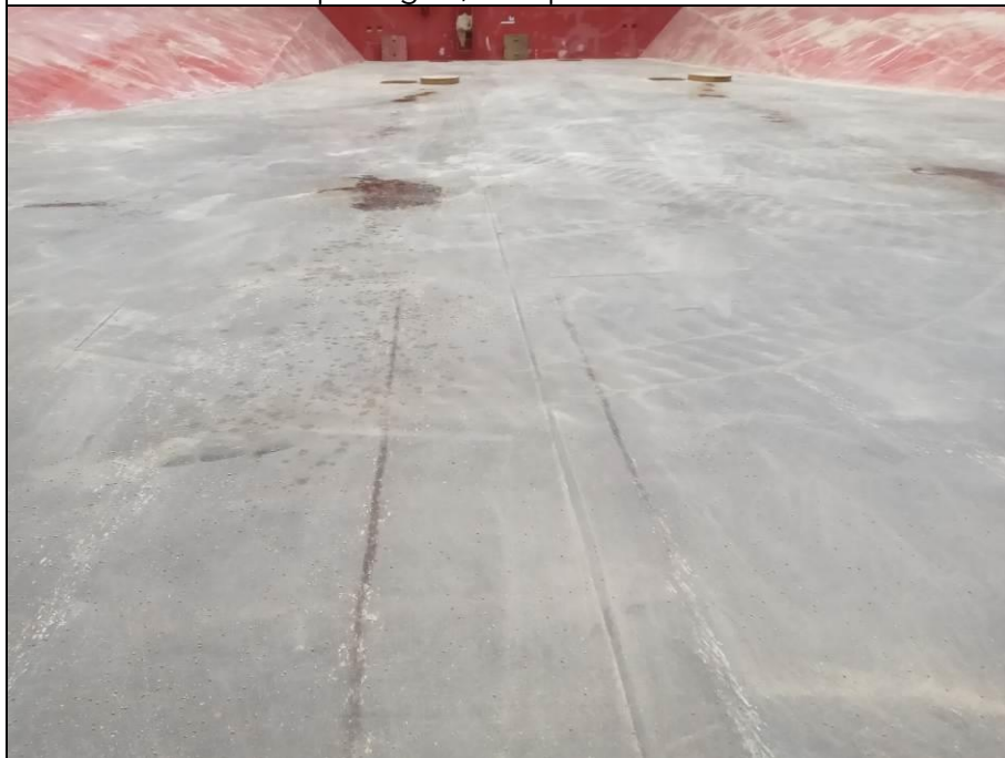
72. Tank top plating with dust.
