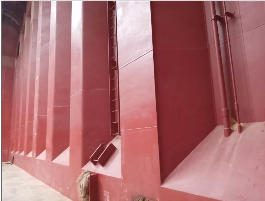
29. Aft bulkhead with paint scratched.
