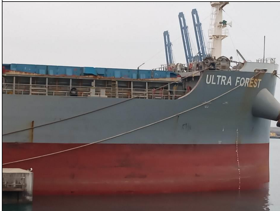
2. Paint scratched and stained were observed at fwd.
