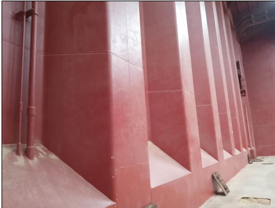
49. Aft bulkhead, with paint scratched and dust.
