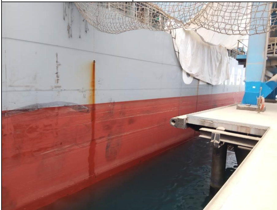
8. Hull with paint scratched and rusty.
