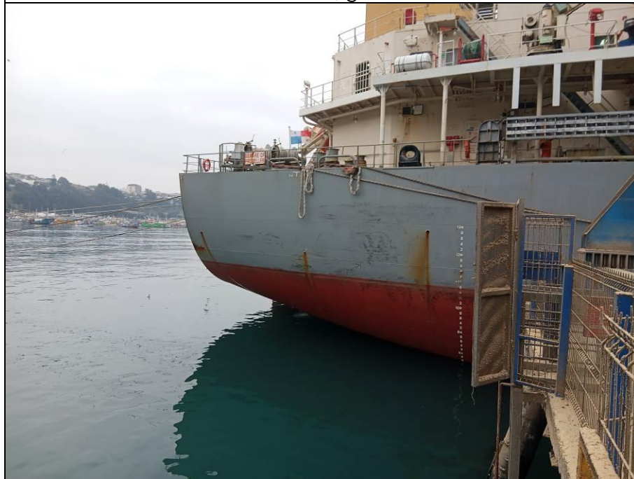
10. Hull with paint scratched & stained.
