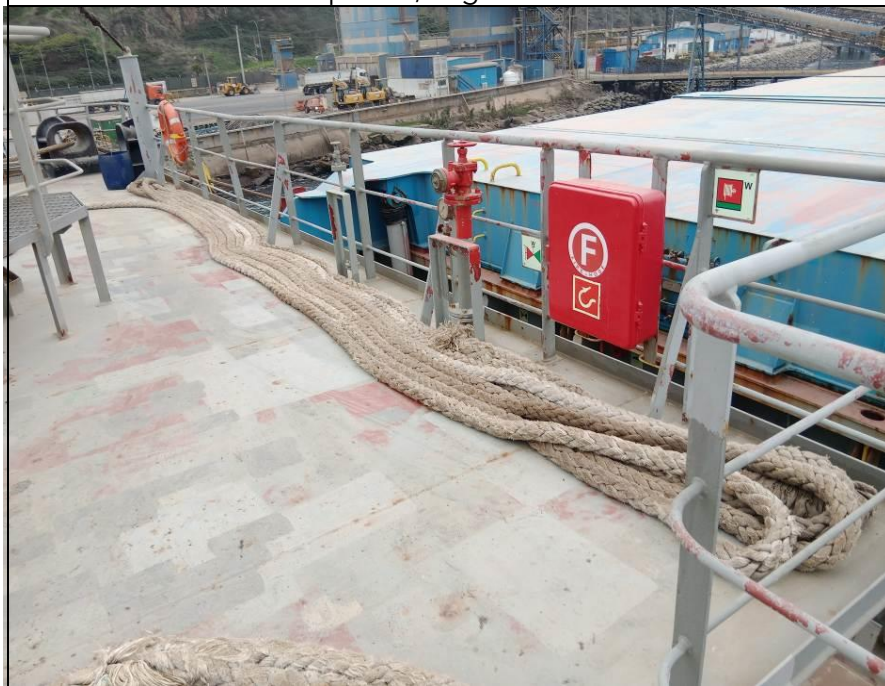
20. Forward mooring lines stained and worn out.
