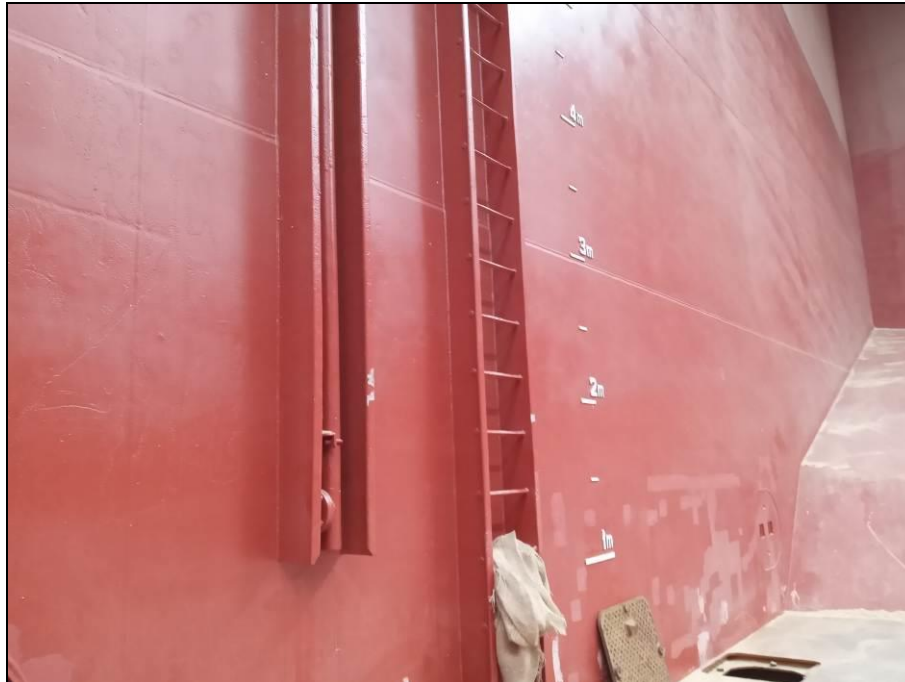
69. Aft bulkhead with paint scratched.
