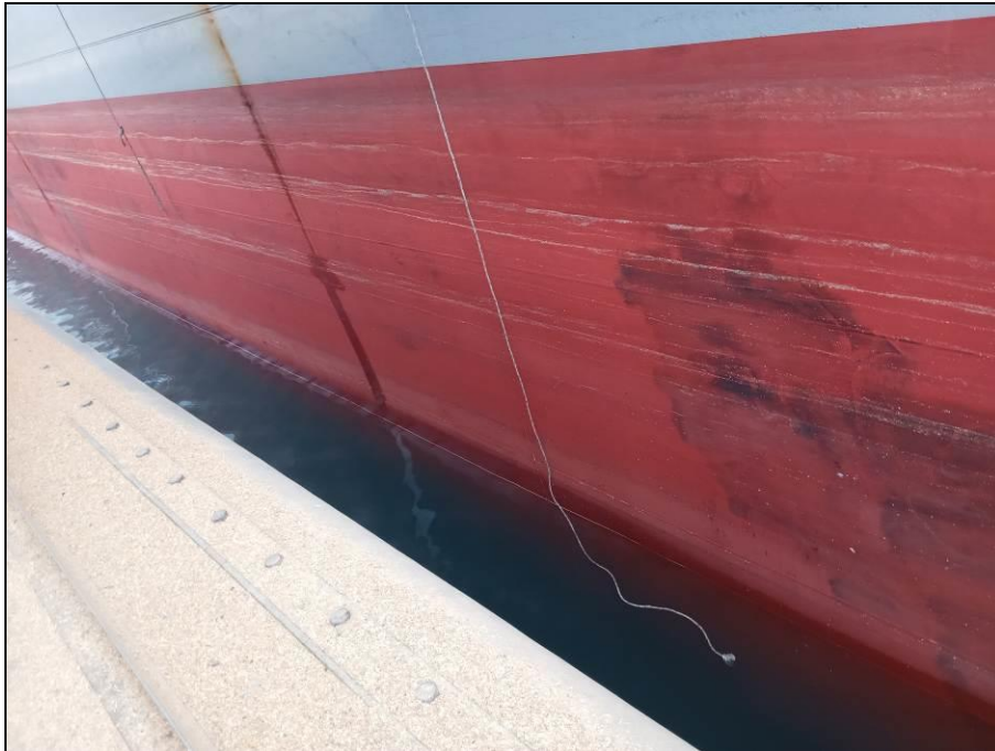
7. Hull with paint scratched.
