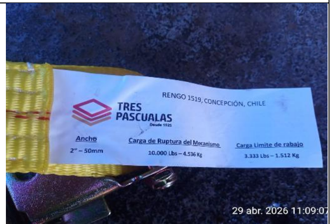
4. View lashing synthetic SWL 4.536 KGS
