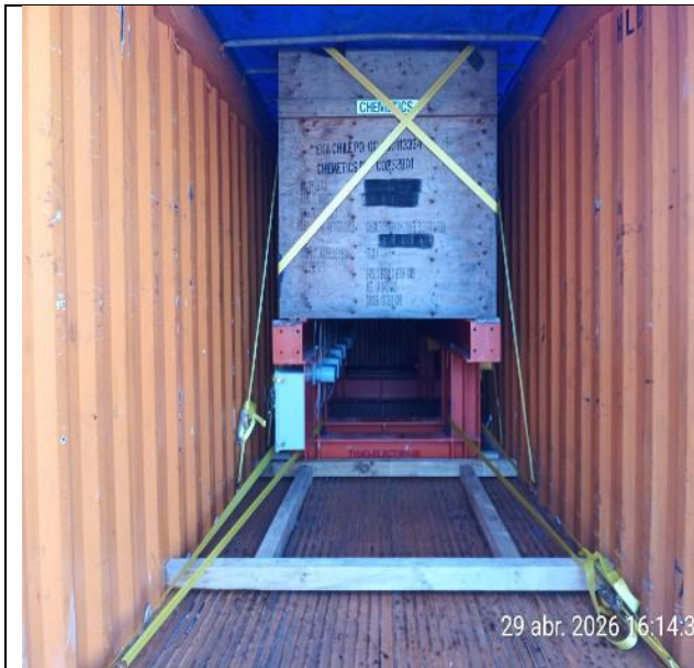
5. Final view of electrolyzer already lashed into container.
