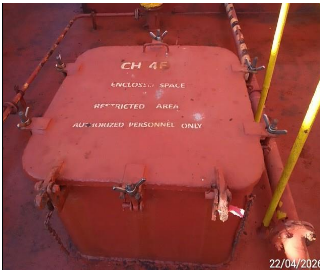
7. Hold Nr. 4, general view of stevedore's access Fwd sealed.
